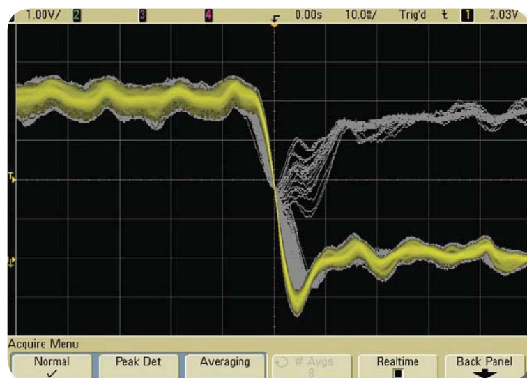
Figure 4: Infrequent event captured by an Agilent 6000 Series oscilloscope.
